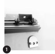
Remove end cap and put Adjustable bracket in place, using 1.5mm (0.06") hex key tighten adjustable bracket in plane (min. 2 per metre/40"). Reinstall end cap.
