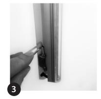
Adjust to required angle and secure with 3mm (0.12") hex key.
